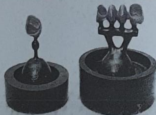
Fig. 12-12 Left, Primary sprue oriented directly toward the wax pattern. Note the spherical reservoir on the vertical sprue. Right, Indirect sprue design showing a horizontal reservoir runner bar that is positioned near the heel center of the invested ring.
